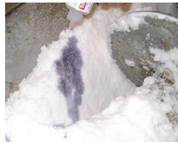
TA 9005-REG identified appropriate technologies and facilitated their transfer—here, a simple test reveals iodine in salt as a dark color (purplish).
