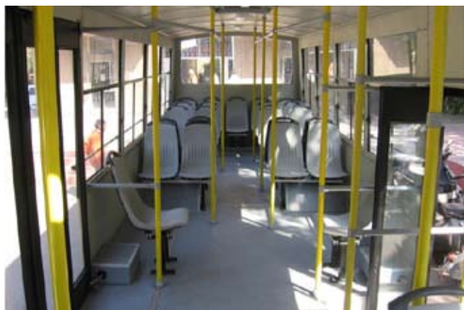
Inside BRT Bus (seen from front to rear: Note the different heights of the doors)
