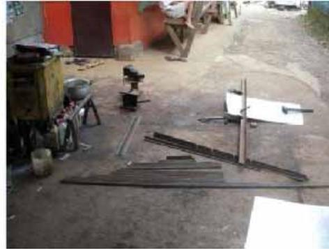
11. Due to the corrosive environment in the island and passengers that are wet with sea water from the beach the metal body of the tricycle easily rusts and wears out quickly. The tricycle body undergo annual repairs or sooner when necessary. Some tricycles use stainless steel bodies that last longer but costs twice than the regular galvanized body.
