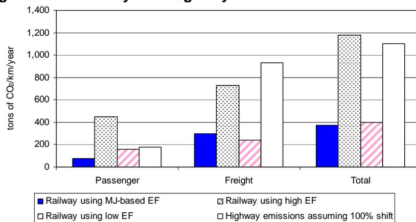
CO<sub>2</sub> = carbon dioxide, km = kilometer, MJ = megajoule, EF=emissions factor, high EF= emission factor equivalent to 130 grams per passenger-km, Low EF= emission factor equivalent to 45 grams per passenger-km.
