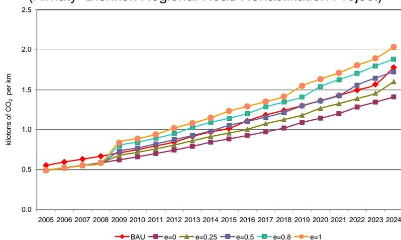
BAU = business as usual, CO<sub>2</sub> = carbon dioxide, e = elasticity of traffic with regard to road capacity, km = kilometer.
