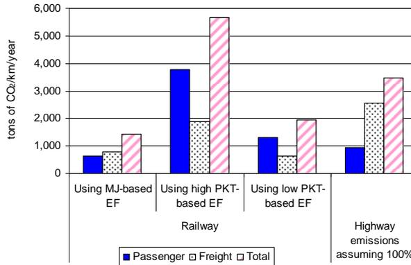
CO<sub>2</sub> = carbon dioxide, km = kilometer, NH = national highway, MJ = megajoule, EF = emission factor, high EF = emission factor equivalent to 130 grams per passenger-km, low EF = emission factor equivalent to 45 grams per passenger-km, PKT = passenger-km traveled.
