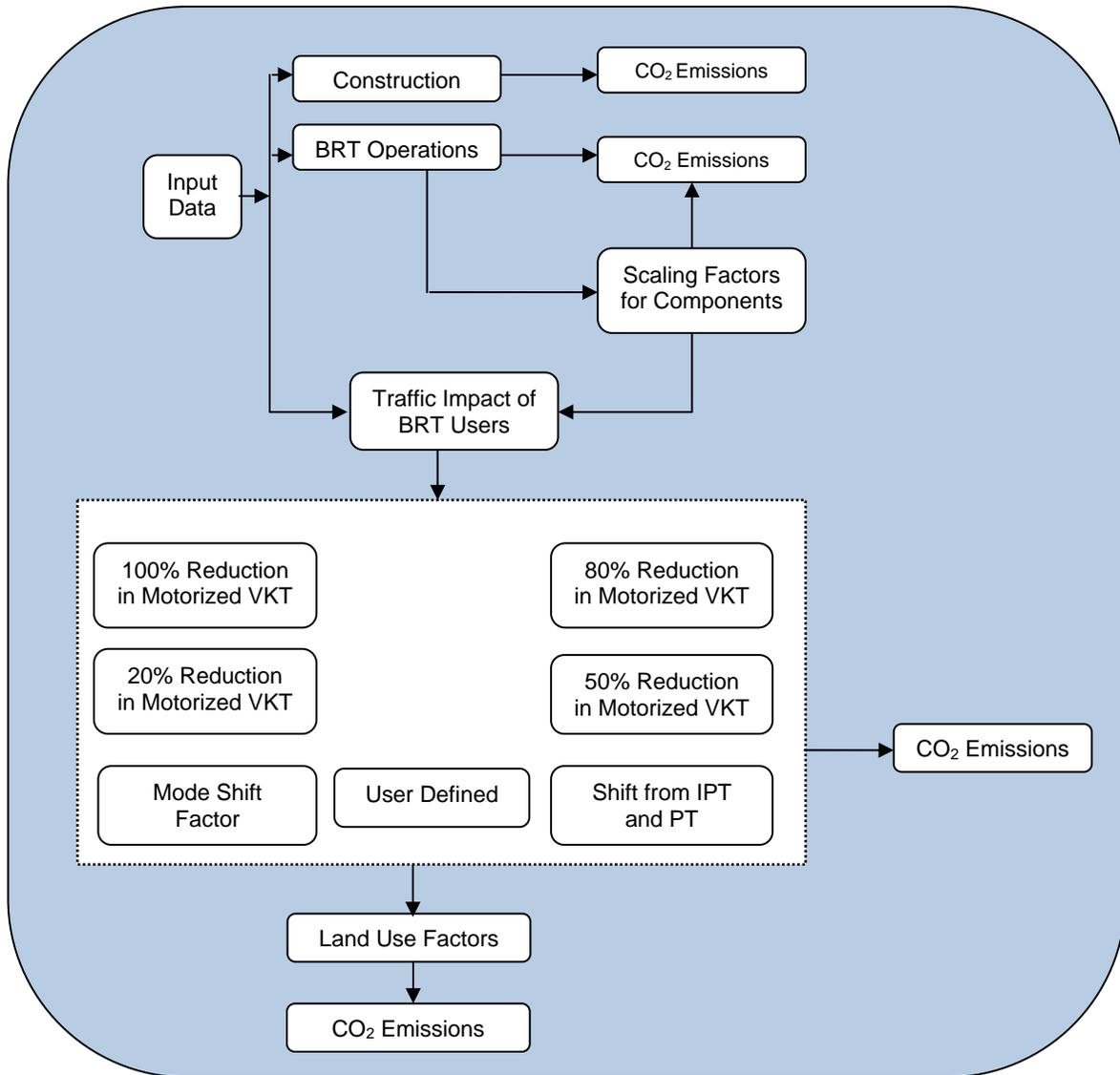
BRT = bus rapid transit, CO<sub>2</sub> = carbon dioxide, IPT = intermediate public transport, PT = public transport, VKT = vehicle kilometer of travel.
