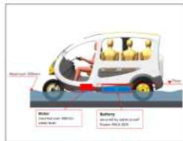
Figure 17. Flood protection
