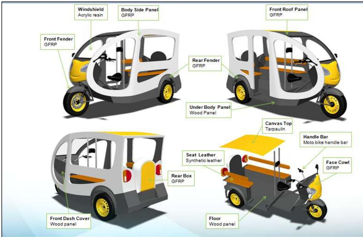
Figure 15. Materials used in the picture models
