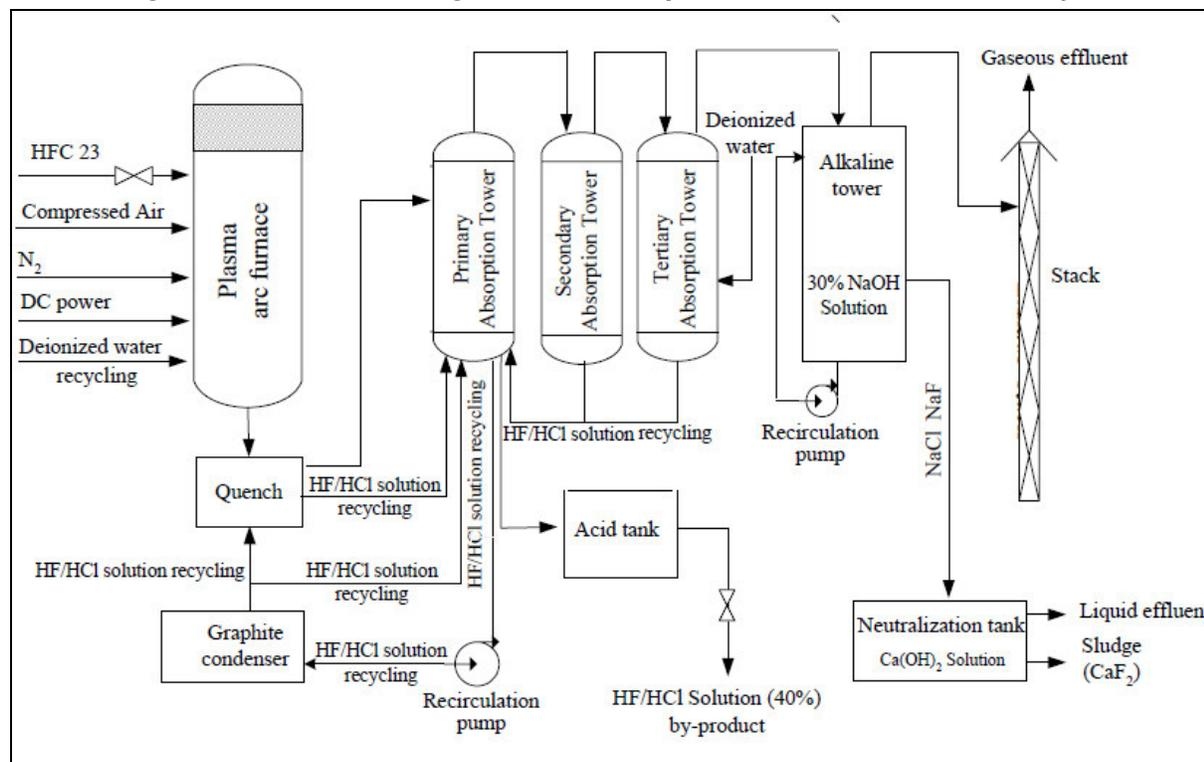
Ca(OH)= calcium hydroxide; DC= direct current; HF= hydrogen fluoride; HFC= hydrofluor carbon; N<sub>2</sub>= nitrogen gas; NaCl= sodium chloride; NaF= sodium fluoride.
