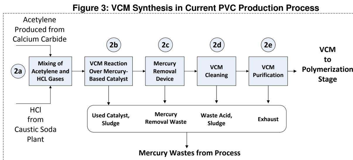
HCl = hydrogen chloride, VCM = vinyl chloride monomer.
