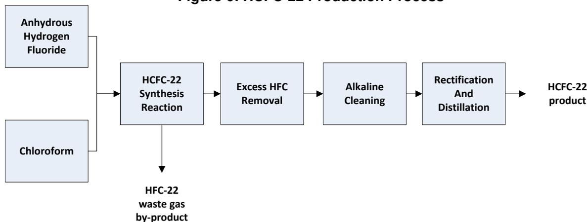
HCFC-22 = difluoromonochloromethane, HFC = hydrofluorocarbon, HFC-23 = fluoroform.
