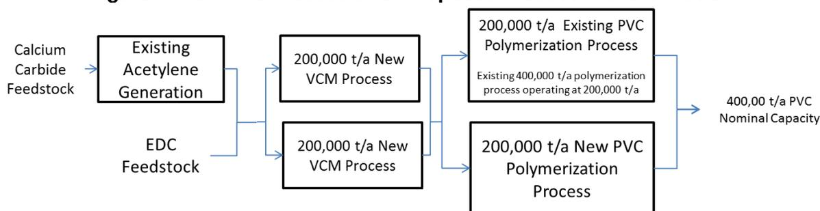
EDC = dichloroethane, PVC = polyvinyl chloride, t/a = tons per annum, VCM = vinyl chloride monomer.
