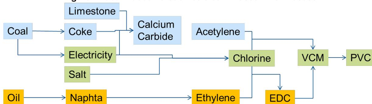
EDC = dichloroethane, PVC = polyvinyl chloride, VCM = vinyl chloride monomer.
