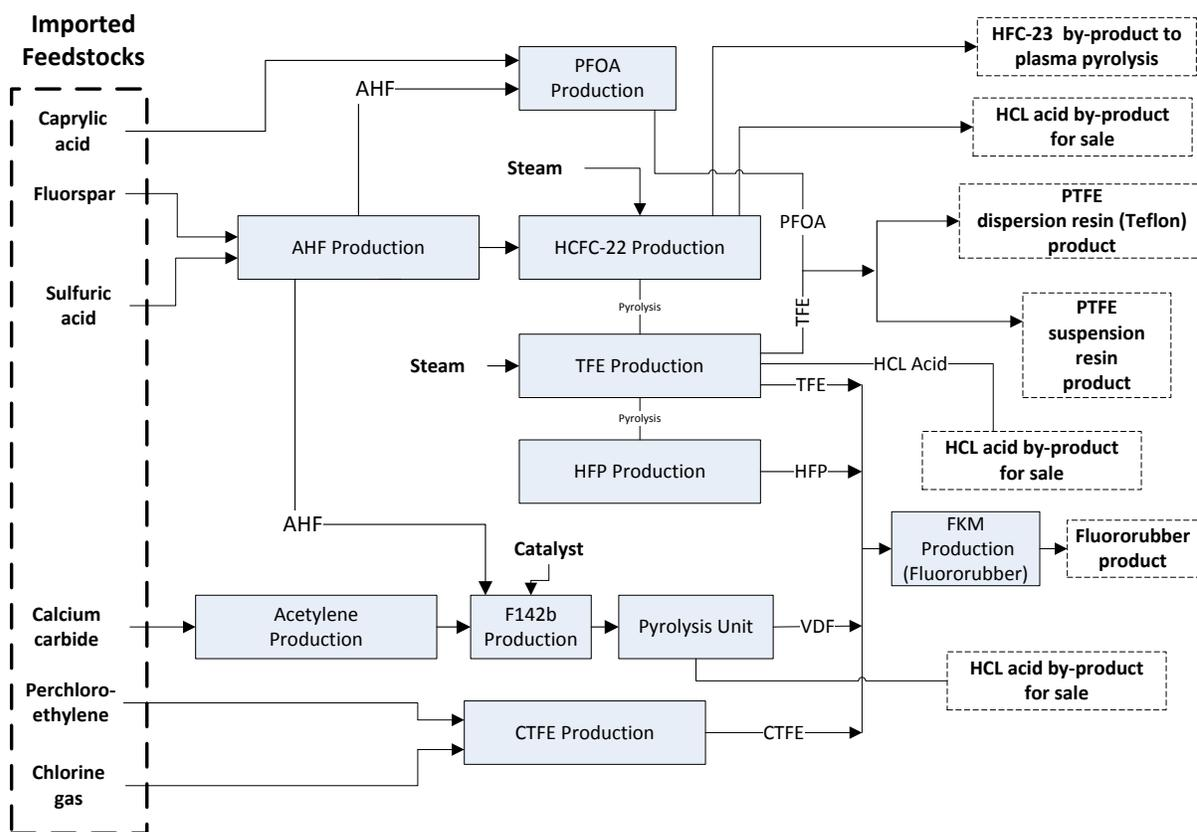
AHF = anhydrous hydrogen fluoride, caprylic acid = octanoic acid, CTFE = chlorotrifluoroethylene, F142b = 1-chloro-1, 1-difluoroethane, FKM = fluoroelastomer, HCFC-22 = difluoromonochloromethane, HCl = hydrochloric acid, HFC-23 = fluoroform or methyl trifluoride, HFP = hexafluoropropylene, PFOA = perfluorooctanoic acid, PTFE = polytetrafluoroethylene or Teflon, TFE = tetrafluoroethylene monomer, VDF = vinylidene fluoride or fluororubber.
