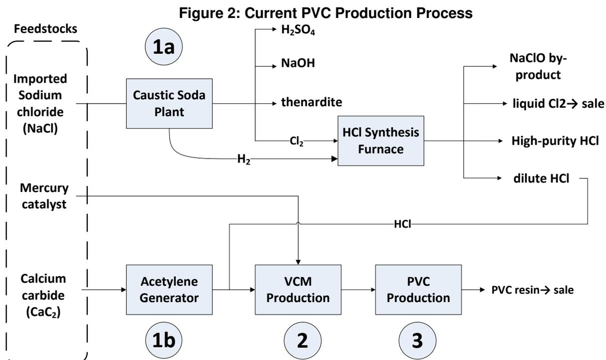
CaC<sub>2</sub> = calcium carbide, Cl<sub>2</sub> = chlorine, H<sub>2</sub> = hydrogen, HCl = hydrogen chloride, H<sub>2</sub>SO<sub>4</sub> = sulfuric acid, NaCl = sodium chloride, NaClO = sodium hypochlorite, NaOH = sodium hydroxide, PVC = polyvinyl chloride, VCM = vinyl chloride monomer.
