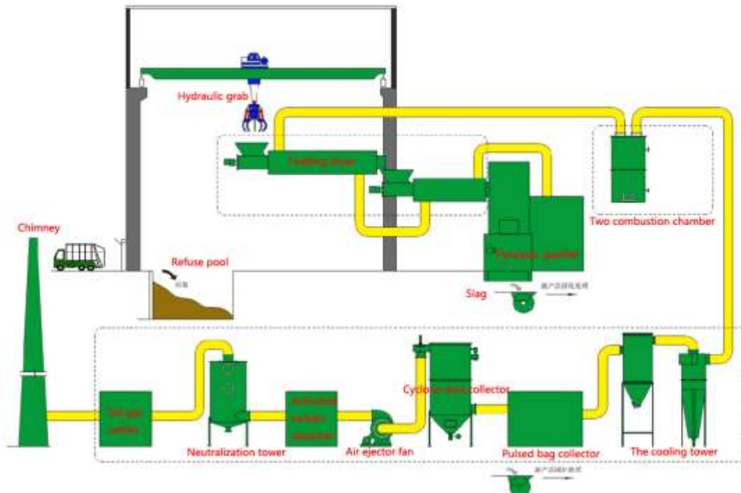
**Figure 4: Process Flow Diagram of Garbage Pyrolysis and Gasification Technology**
