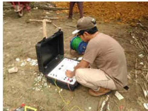
*Implementation of geoelectrical survey at GL-3***Figure 3-4** Implementation of geoelectrical survey at investigation area
