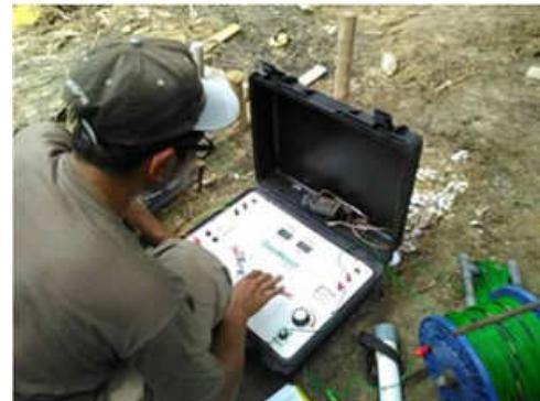
*Implementation of geoelectrical survey at GL-2*
