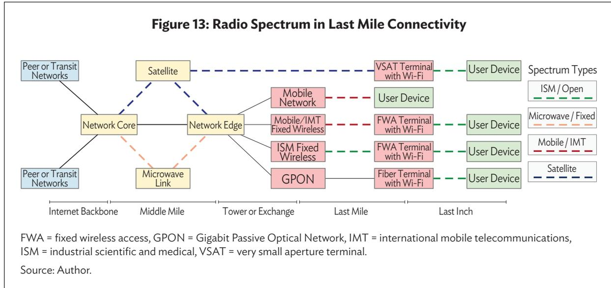
Three primary radio spectrum bands are used in last mile communications to service the four roles illustrated in Figure 13. They are summarized here and explained more fully in Appendix 1.
