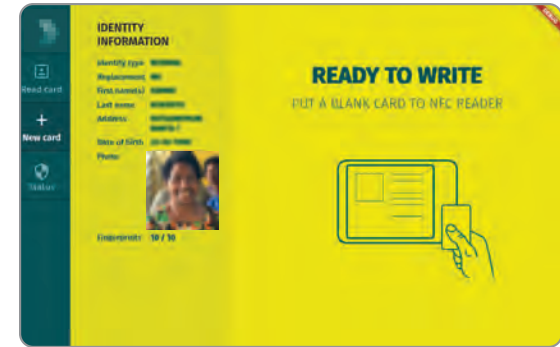
(8) The ID is ready to be written on the card. Agent places blank card near the near-field communication (NFC) antenna on the device, and the data is transferred to the card.
